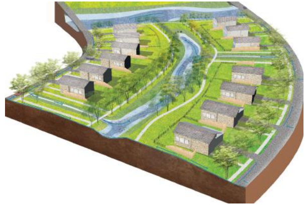
Illustration 13. R. G. Miller Engineers, Inc. and Asakura Robinson, Inc. / Feasibility study rendering of natural drainage residential development (or low impact development) with creek system and linear detention, infiltration, and stormwater quality features.
